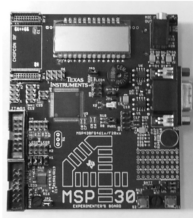
Figure 2.4 - MSP430FG4618 experimenter board. The LCD screen shown displayed the output frequency of the ultrasound transducer.
